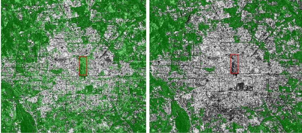
Figure 65. Beijing Result, Left: From the original Pavia method, Right Improved urban extraction using the contrast enhanced SAR data.
