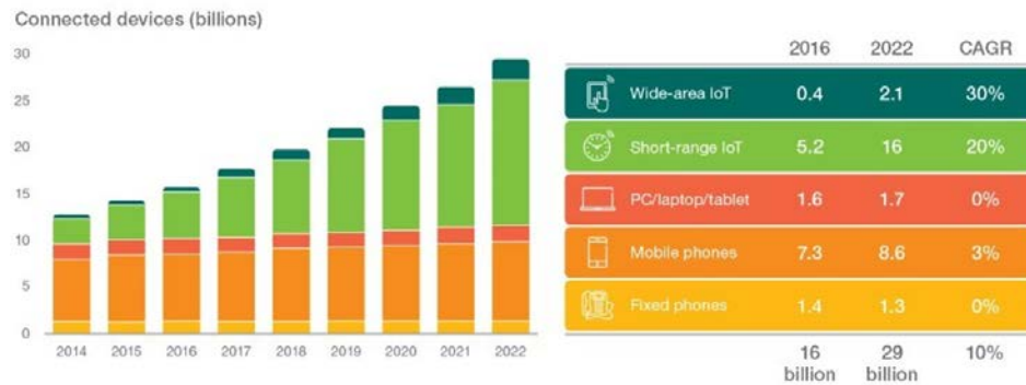
Figure I.6: Connected Devices growth forecast in next years: The exponential increase in connected devices will seriously affect the Network Structure.
