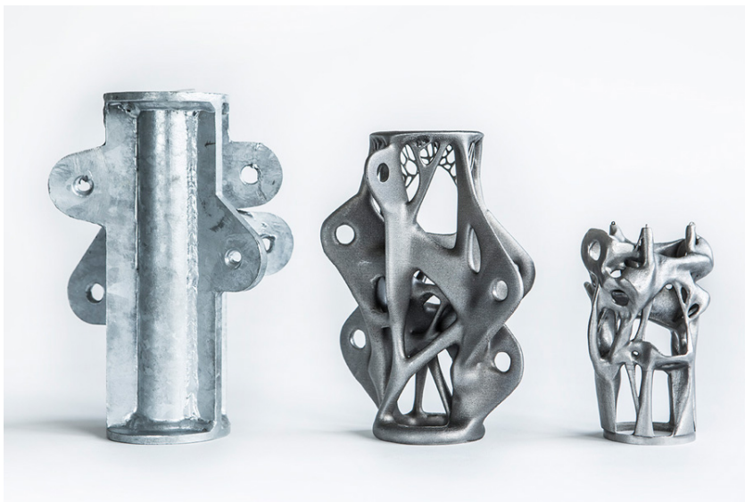
Figure 1.2. 3D Printing steel joints designed by the Arup's team: the three structural elements (nodes) are all designed to carry the same structural loads and forces (reproduced from ARUP [2014] ).
