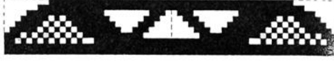
Figure 5.4. Example of checkerboard pattern in simply supported beam, figure taken from Sigmund and Petersson [1998b] .
