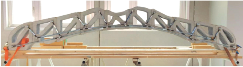
Figure 4.9. 3D printed RC beam with a variable curved cross section.
