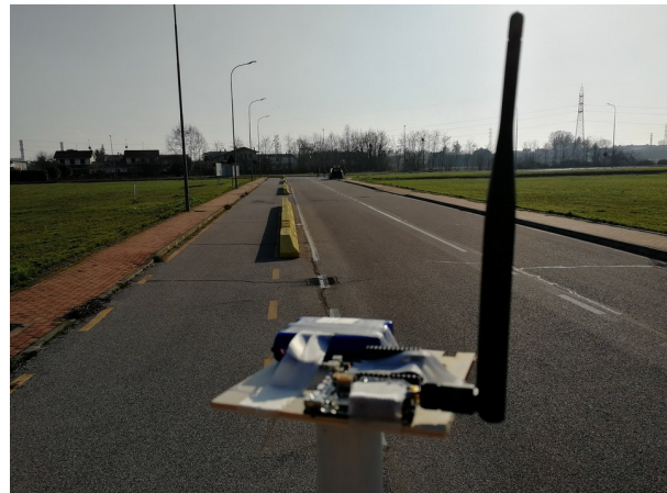
Fig. 3: A view of the experimental setup used for channel characterization measurements of the outdoor environment
