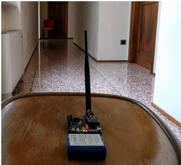
Fig. 2: A view of the experimental setup used for channel characterization measurements of the indoor environment
