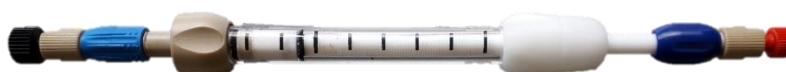
Figure 2-11: PolyHIPE-based monolithic column achieved by the in-situ polymerization of the corresponding emulsion in an Omnifit® empty glass column.
