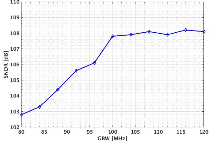
Figure 4.8: SNDR as a function of GBW for the Incremental OTA.
