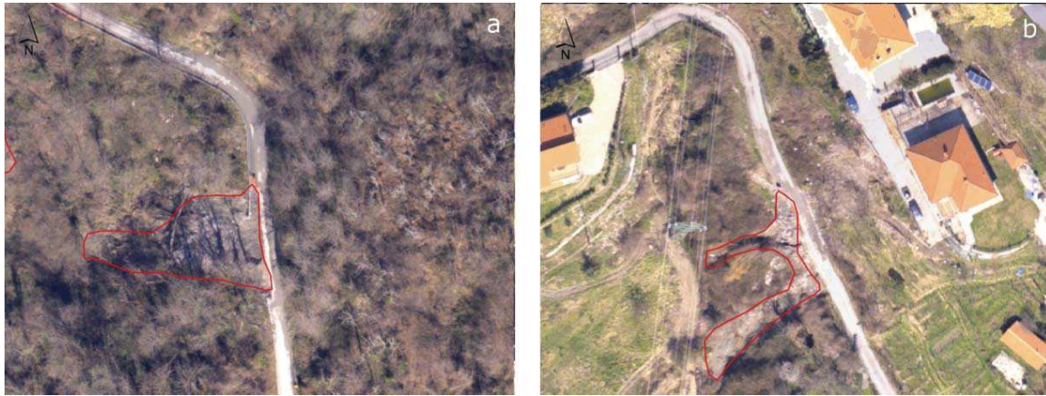
Figure 8. Shallow landslides interaction with road network.
