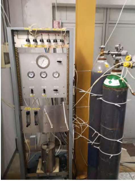
Figure 3.19: Mixer station used for the test. Green bottle is Argon while the grey one is carbon dioxide.
