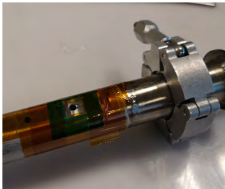
Figure 5.24: Close up of the wire chamber. The holes are made to let particles in, a thin polyethylene layer is placed to let alpha particles in and assure the gas tightness.
