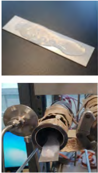
Figure 5.7: Detail of the stainless steel plate where the glue is deposited; after being dried up the plate is placed inside the out-gassing tube. The gas flushing here becomes contaminated before entering the detector.
