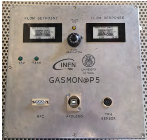
Figure 3.30: Front panel of the controller box. Displays show the set flux and the measured one, the potentiometer regulates the set flux. Connectors to the MFC, PC and the environmental sensor are shown at the bottom.
