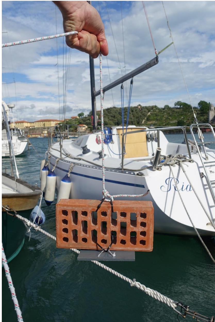
Figure 2.3 PVC panel attached to a brick (as weight) and to a rope: this is the standardized experimental unit of the SERC protocol.
