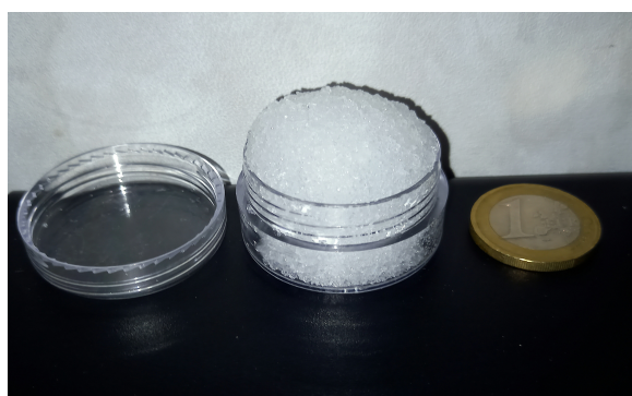
Figure 3.3: Example of a container used to investigate the properties of the sodium polyacrylate. The picture shows the mixture of powder and water at the end of the gelling phase. Each container was 5 mm in height and 20 mm in diameter.
