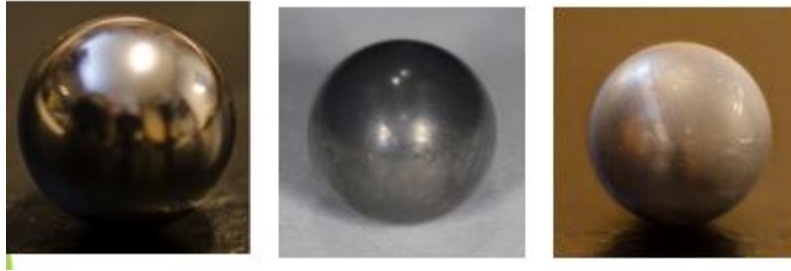
Figure 51: A new bearing ball compared with step 1 and step 2 worn balls (respectively from left to right).
