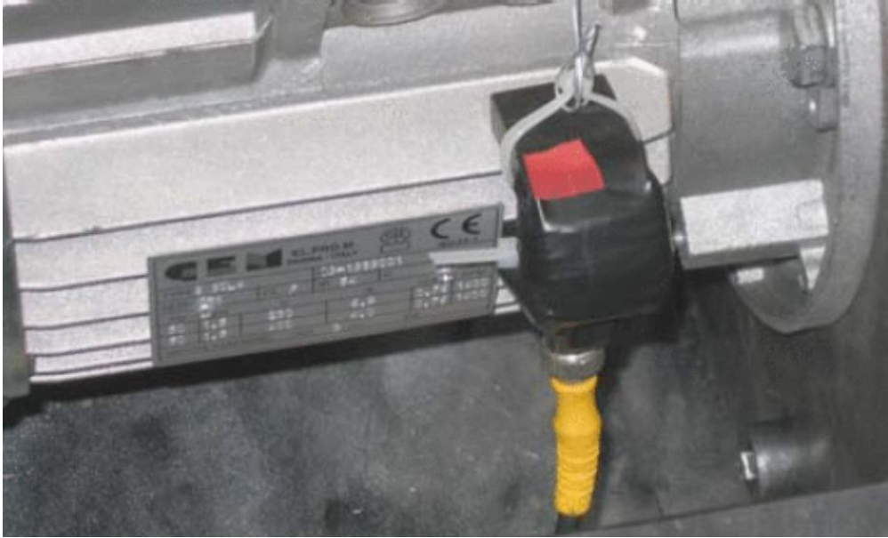
Figure 11: C-shape magnetic-core coil probe [35]
