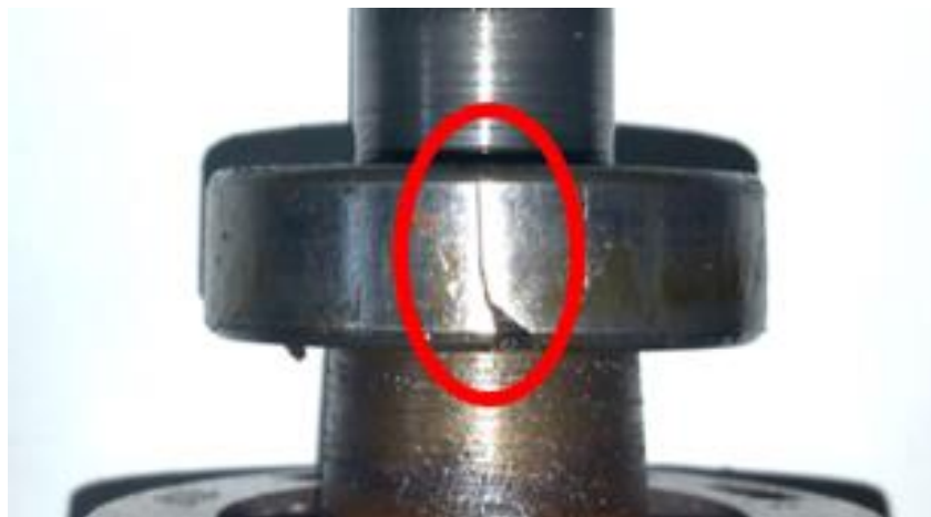
Figure 63: the damaged NSK6205Z bearing.
