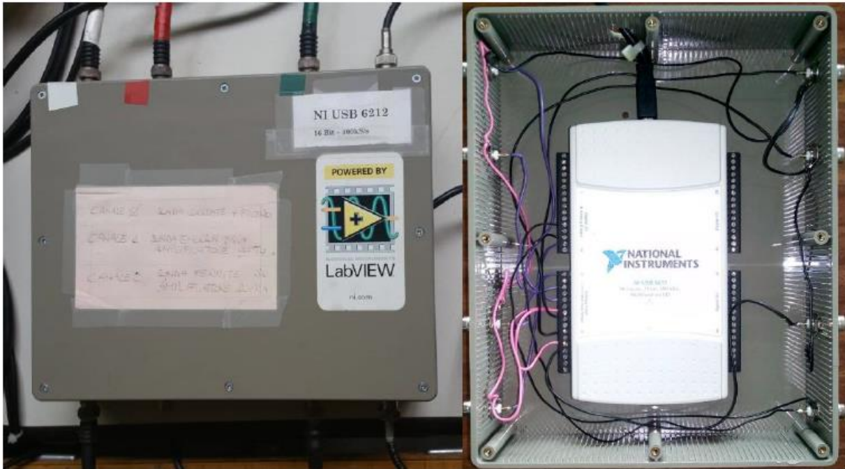
Figure 40: NI USB 6212 DAQ board and plastic case protection used.
