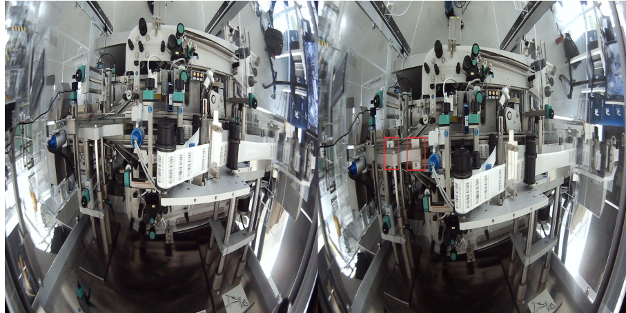
FIGURE 3.1: Example of a machine to be monitored. Left: clean machine. Right: machine with two cases interlocked in line. We have highlighted the cases with two red bounding boxes. Images are juxtaposed to highlight the spatial shift.
