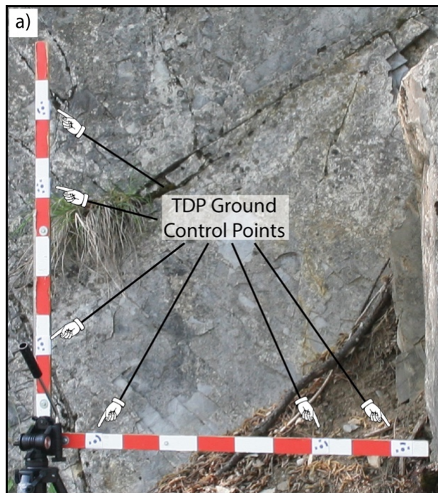
Fig. 4 Example of Ground Control Points (GCPs) of the photographic scale. The accuracy of the GCP position is of 1mm.
