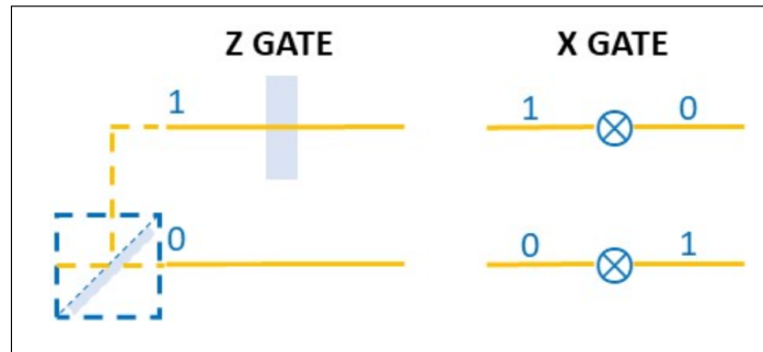
FIGURE 7.26: Idealized design of Z and X gates on a dual-rail-encoded qubit. In order to avoid a confusion between this representation and a two-qubit circuit - where the parallel lines stand for different registers -, in the first example we added the beam-splitter and two outgoing beams (dashed lines).
