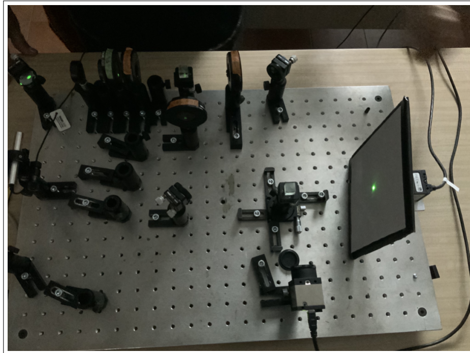
FIGURE 7.35: Experimental setup for the implementation of Deutsch's algorithm
