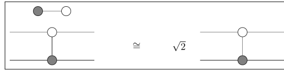
FIGURE 4.15: Two diagrammatically equivalent variants of the CNOT gate
