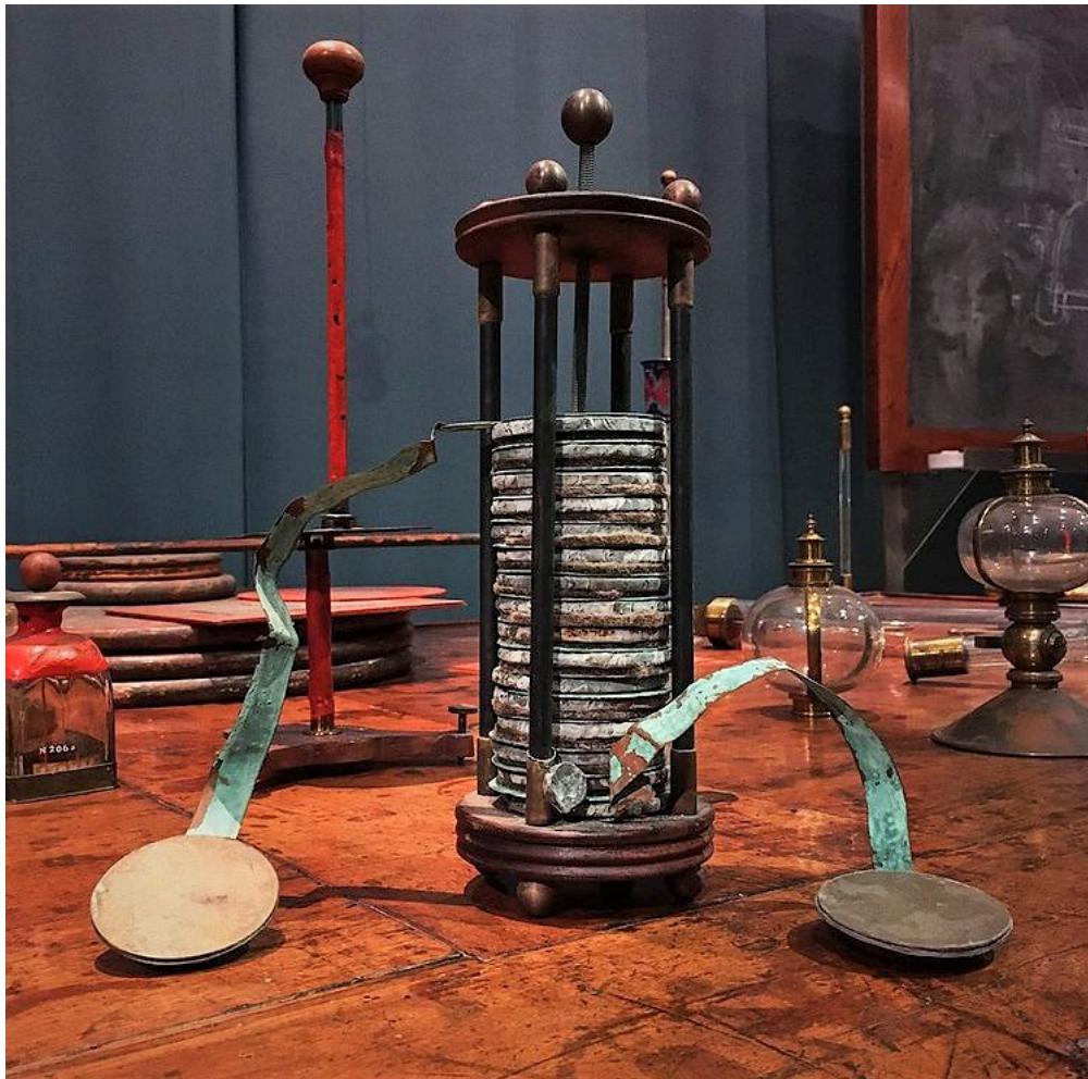
Figure 2.1: Example of the battery built by A. Volta, preserved in the Museum of Electrical Technology, Pavia, Italy.
