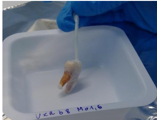
Figure 5.2.3.4.1. Example of a tooth that has been wrapped in parafilm, leaving only the lower part of the root exposed. Note the tail of parafilm present to allow for easier handling of the tooth
