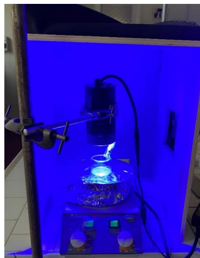
Figure 9.2. Irradiation system used in this work: A 40 W Kessil lamp (with emission centered at 427 nm) is held three centimetres above the glass reaction vessel which was stirred gently for 24 hours. A fan is placed on the right of the reaction vessel to avoid any heating of the solution.
