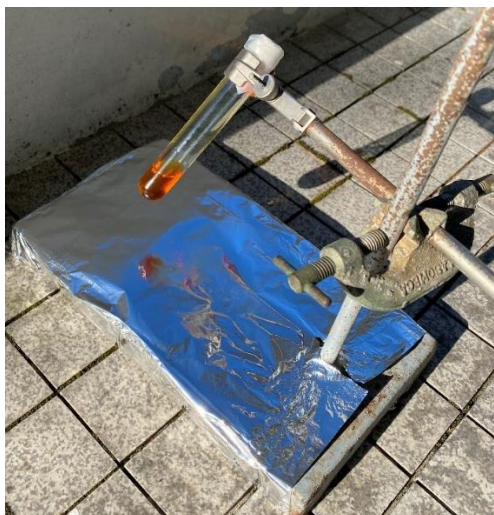
Figure 8.14. The vessel containing the arylazo sulfone and the styrene under direct sunlight exposition with an aluminium foil beneath it.
