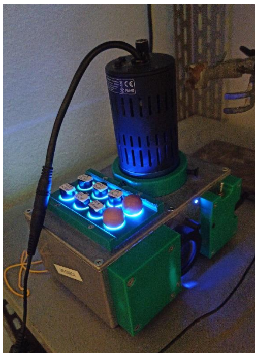
Figure 6.6. Photochemical set-up employed for the coupling reaction of arylazo arylsulfones.
