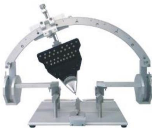
Figure 2.5| Eckhorn Matrix. Multi-electrode array system mounting up to 16 independent electrodes in a matrix 4x4 with inter-electrode distance of 100 \mu\text{m} .
