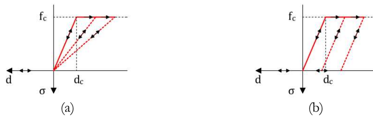
Figure 7.2: Constitutive laws for masonry at the end interfaces of the macroelement: (a) Penna et al. (2014) and (b) Bracchi et al. (2021).
