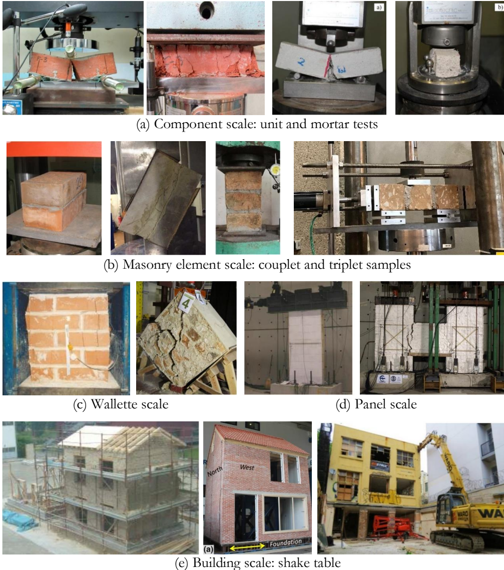
Figure 2.14: Examples of masonry tests at different scales: (a) Ganbaatar et al. (2022) and Marastoni et al. (2016); (b) Churilov and Jovanoska (2013) and Thaickavil and Thomas (2018); (c) Budiwati (2009) and Milosevic et al. (2013); (d) Magenes et al. (2008) and Graziotti et al. (2012); (e) Magenes et al. (2010), Miglietta et al. (2021), and Hogan et al. (2008).
