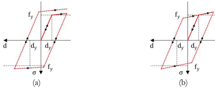
Figure 7.5: Elasto-plastic constitutive laws for strengthening/reinforcement at the end interfaces: (a) isotropic and (b) kinematic hardening.
