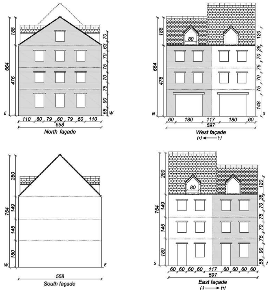
Figure 4.1: Dimensions of the half-scale masonry building aggregate specimen.
