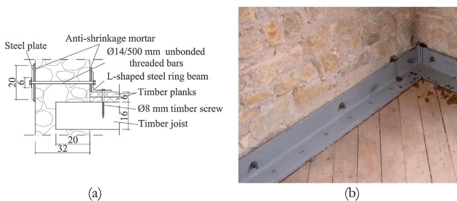
Figure 3.6: Building 2, retrofit at the first-floor level: (a) structural detail of the wall-to-diaphragm connection; (b) steel-angle ring beam at a building corner and 45-degree-oriented additional timber planks. Units of cm.
