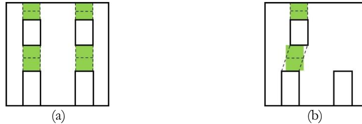
Figure 2.8: Examples of discretization criteria for masonry spandrels in case of (a) regular and (b) irregular opening distribution (Lagomarsino et al. , 2013).
