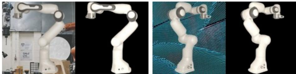
**Figure 10.4:** Examples of two synthetic images, along with their ground truths, for the training of the CDA.
