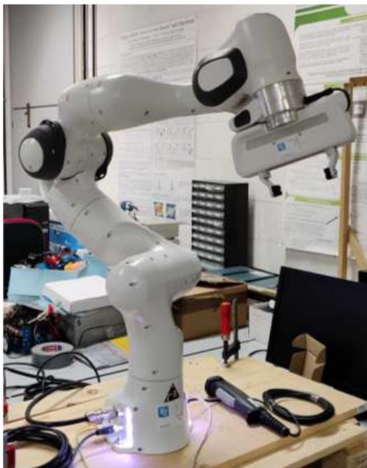
**Figure 4.1:** Example of open-chain manipulator with seven revolute joints, eight links, and a gripper as end-effector.
