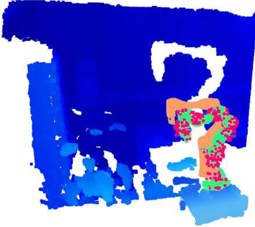
**Figure 10.8:** Result of the HE calibration process. Depth points from the camera are in blue and green. The orange 3D model represents the first pose estimate, while the red points the result of the ICP algorithm.
