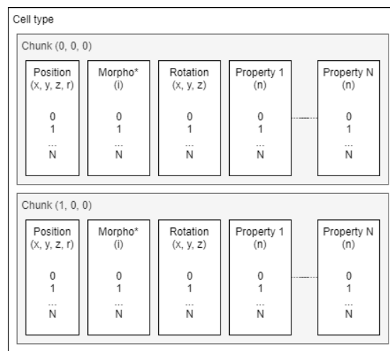
Figure 2.8: The placement data model. Each inner white square denotes a dataset object, with in parenthesis the data per record in the set. All datasets are parallel to each other, e.g., position 1 is associated to rotation 1. (*) A MorphologySet : A set of morphology names, and a multiset containing the index of the associated morphology name per cell. The morphologies themselves are stored separately by the MorphologyRepository . The rotations are similarly wrapped by a RotationSet which lets users use the convenient scipy.Rotation per item in the dataset.
