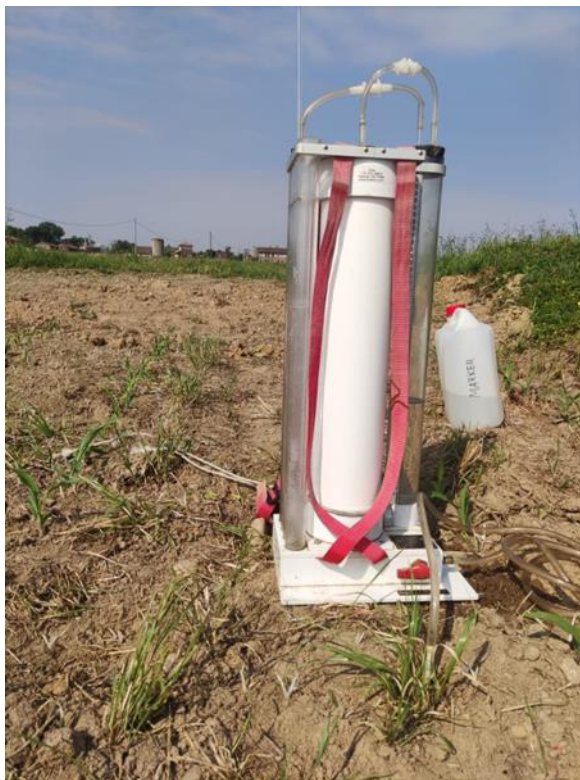
Figure 6: amoozemeter during fieldwork
