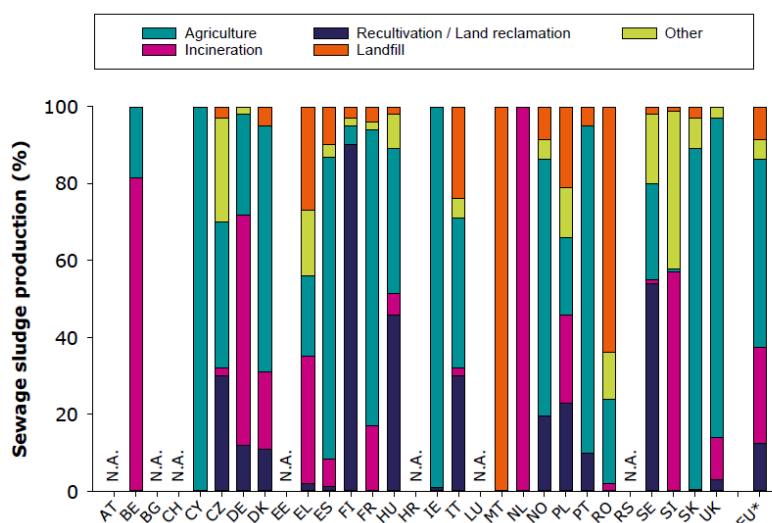
Figure 5- Sewage sludge usage in European countries (Years 2013-2015). Data extrapolation is not available for Austria, Bulgaria, Croatia, Denmark, Ireland, Serbia and Switzerland.
