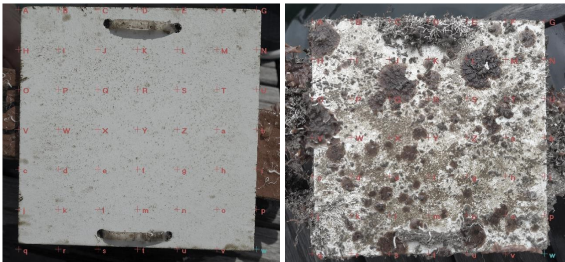
Figure S16. Uniform gridded (7 x 7) design showing the point display for image analysis in the software CPCe (Coral Point Count with Excel extensions) (Kohler & Gill, 2006). Based on a code created for the purpose, specific entries can be assigned to each point. For the analysis of coverage through time, the entries cover , bare or slime were employed and data was then used to calculate the percentage coverage of each plate per month. The picture on the left belongs to a BC treated plate after one month of submersion (month of June), mostly covered by a fine slime. The picture on the left belongs to the same plate after three months of submersion (month of August).
