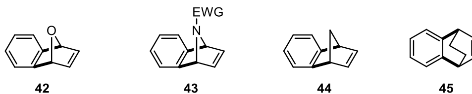
Figure 8: carbo- and heterocycles fused with benzene ring achieved via aryne [4+2]-cycloaddition
