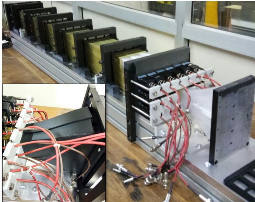
Figure 4.8: Sixteen PMTs are mounted on the module. Patch panels and electronic boards are not yet mounted. The inset image shows the isolation of central tower fibres from PMT cabling.
