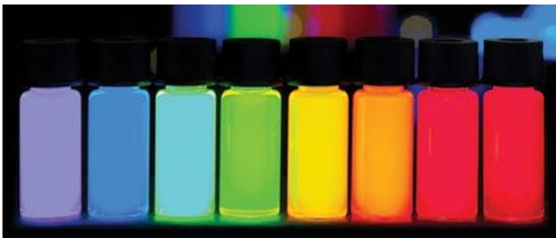
Figure 1.1 Colloidal suspensions of semiconductor quantum dots under UV illumination. Adapted from ref [28].
