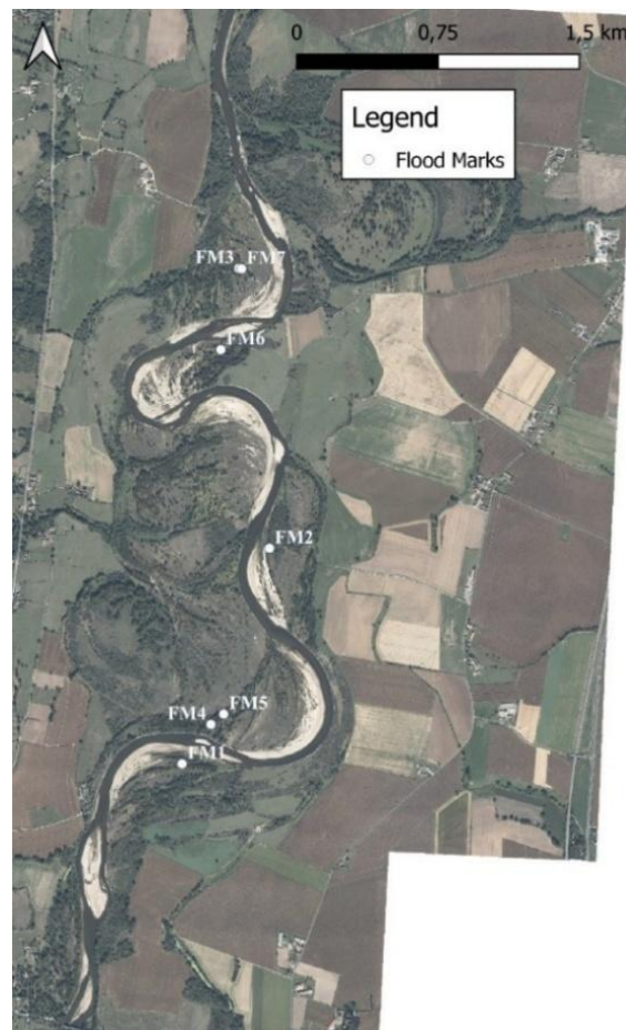
Figure 9.5 Location of surveyed flood marks along the Allier River study reach downstream of the Châtel-de-Neuvre hydrological station.
