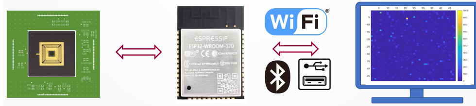
Figure 2.14. A conceptual connection overview of the microcontroller as the interface between the sensor and the PC.
