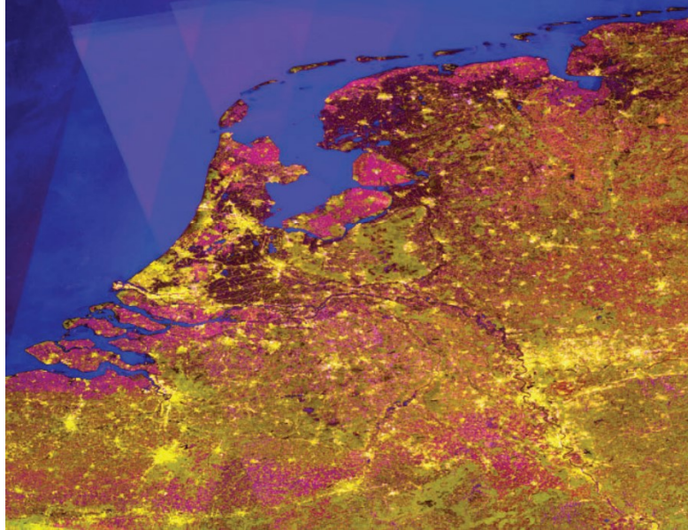
FIGURE 2.5: False color composite of average SAR backscatter (red), minimum SAR backscatter (green) and standard deviation (blue) for the Netherlands. Dataset: Envisat ASAR Wide Swath Mode. Image source: [43].
