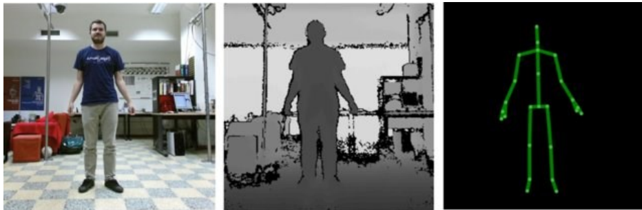
Figure 2.8: The three different types of Vision-based data, starting from left to right: RGB data, Depth map data, Skeleton data.
