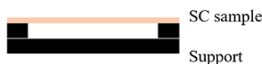
Figure 1. Illustration of the support used to place the SC during the irradiation in the Q-Sun Xenon Test Chamber.
