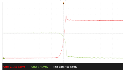
Figure 2.30: N2-1 turn on (a) and turn off (b) at 4 A, 25 °C
