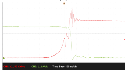
Figure 2.37: N3-1 turn on (a) and turn off (b) at 10 A, 150 °C
