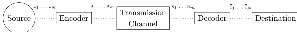
Figure 2.2: A schematic representation of a communication setting. A discrete source generates a sequence of N symbols that are the input of the encoder, used by the sender to generate a string of bits that represents a compressed version of the original message. Then a transmission channel is used to convey the latter to the receiver, that finally decodes the message.
