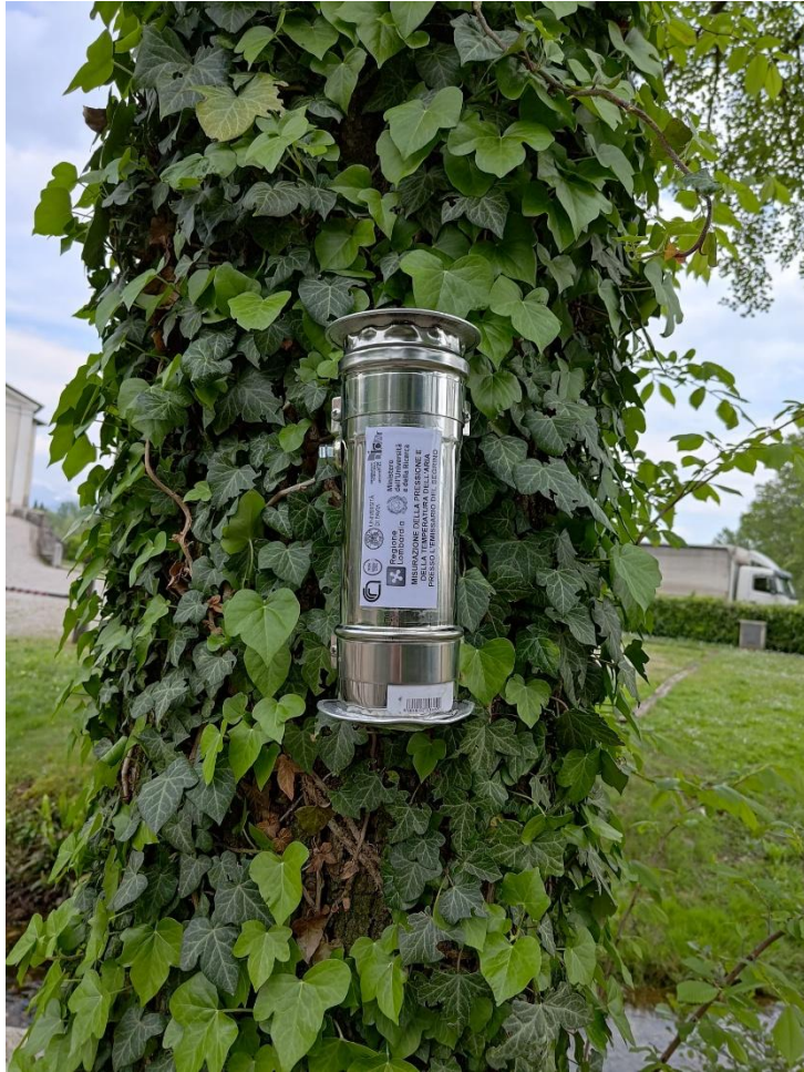
Figure 18. HOBO monitoring device installed next to the Lake Segrino outlet stream for measuring reference atmospheric pressure needed to convert the water pressures measured by the stream gauges into levels, in addition to air temperature.
