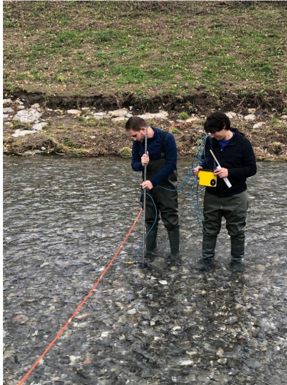
Figure 15 . Measurement of velocity with the Valeport Model 002 current meter along the verticals at the Lambrone section.
