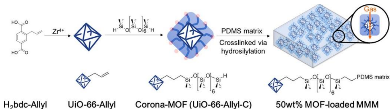
Figure 3.3. MMMs prepared from corona-MOFs and a PDMS matrix. The corona is covalently connected to both the surface of the UiO-66-allyl particles and the PDMS polymer matrix via hydrosilylation From ref. [14].
