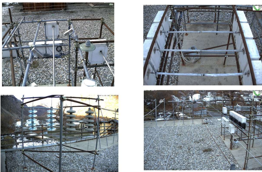
Figure 3.9 – webcam image of the WILD station on a nice winter afternoon (top-left and right 12 slots for 75cm samples, bottom-left: insulator testing , Bottom-right:15m wires)
