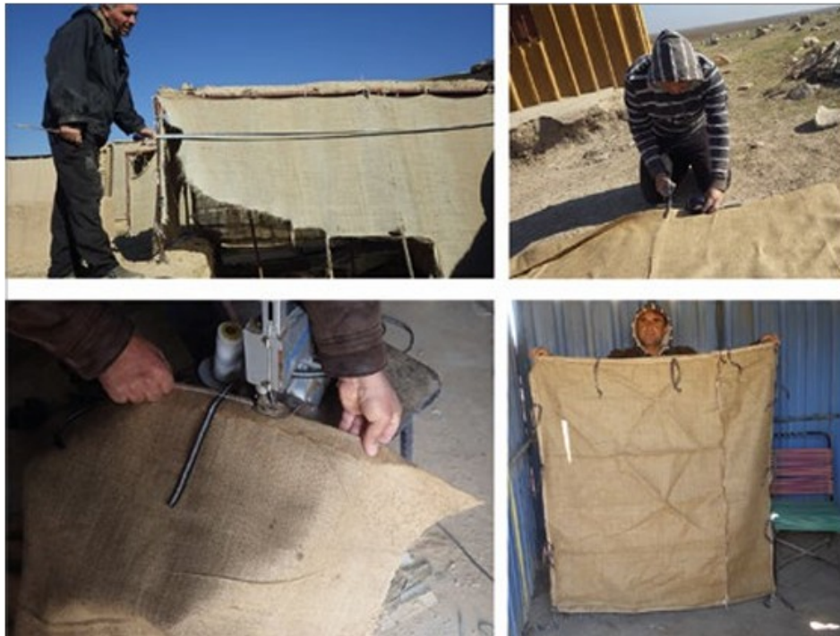
Figure 60: The new curtains being made: top left, taking measurements of a torn curtain to be replaced; top right, designing a new curtain; bottom left, sewing a new curtain; bottom right, a completed curtain before installation. Source: Buccellati. 2019, 194.
