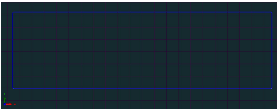
FIGURE A.1: Visualization of the G-code to generate a rectangle. The blue lines depict the filament paths.
