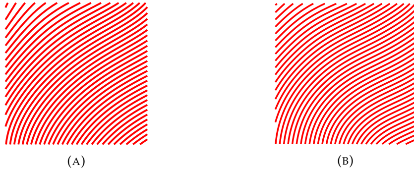
FIGURE 3.10: Comparison of the optimized filament paths from 1-by-1 and 4-by-4 patches under the same initial conditions. (A) Centerlines of the optimized filaments for 1-by-1 patch with c_f/c_{in} = 0.63 . (B) Centerlines of the optimized filaments for 1-by-1 patch with c_f/c_{in} = 0.60 .
