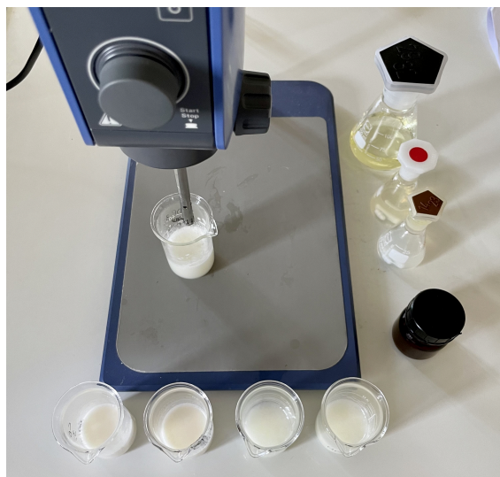
Figure 62. Image of different emulsions prepared by using various concentration of pectin (1%-3% w/v) and sunflower oil (35%-60% w/v).
