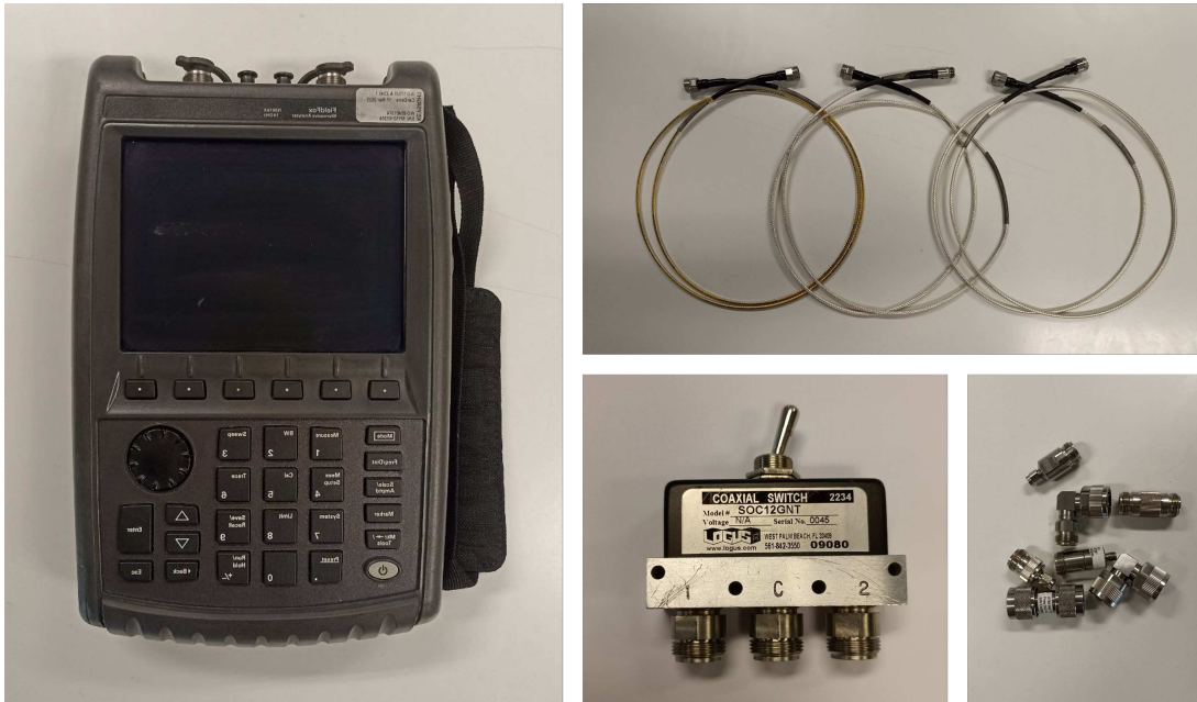
Figure 2.3: Equipment for the setup, from the left, top: Field Fox VNA; coaxial cable with N-type output; mechanical RF switch up to 12 GHz; some of the RF adapters used to connect the antennas.
