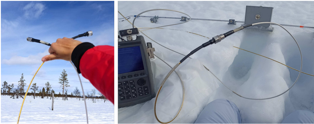
Figure 2.9: Two step of calibration when the antennas are not connected.
