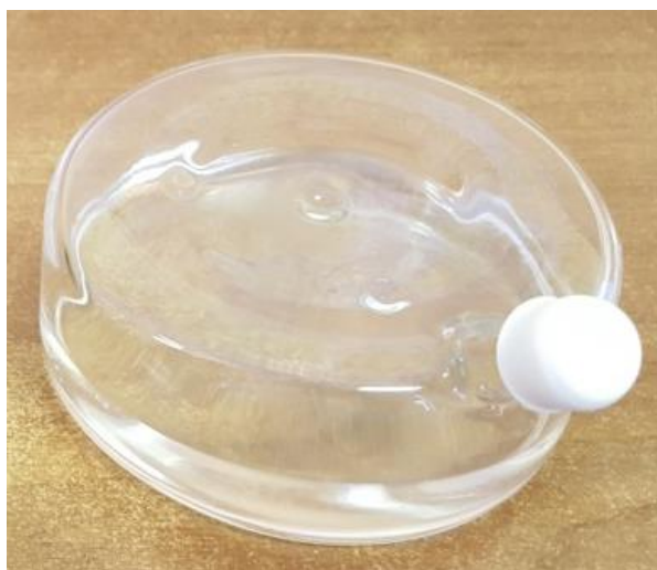
Figure S.3.1 Pyrex reaction vessel used in this work
