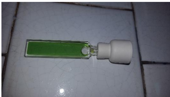
Figure 4.S.3 Cuvette containing the reaction mixture before irradiation
