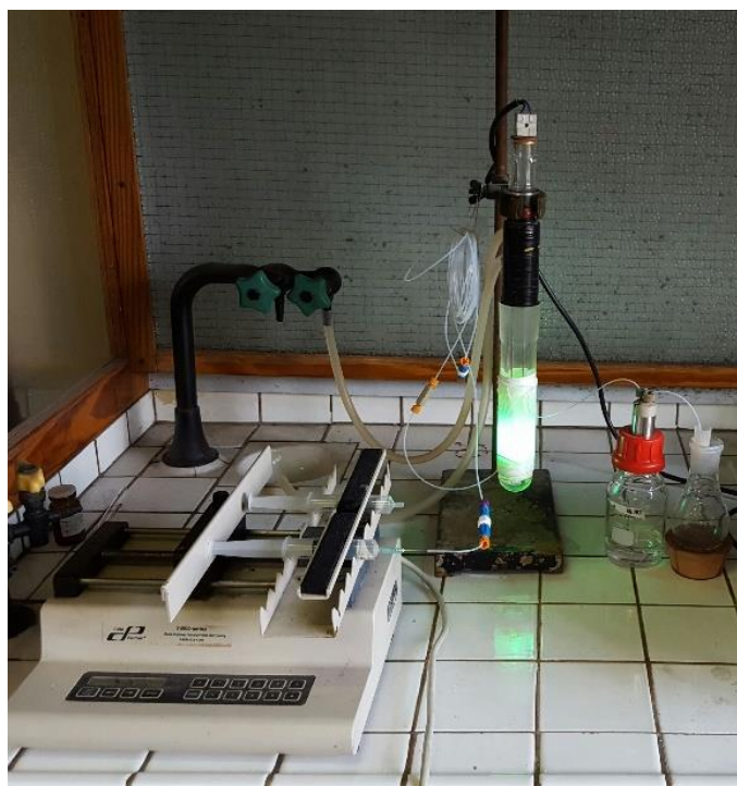
Figure 3.2 Picture of the flow reactor used in this work, equipped with a syringe pump.
