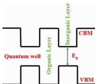
Figure 12 Schematic representation of quantum well structure of a 2D perovskite. Reprinted with permission from ref. [13] Copyright © 2019 WILEY-VCH Verlag GmbH & Co. KGaA Weinheim.
