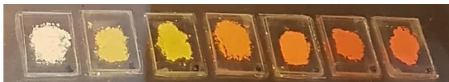
Figure 29 Samples of the solid solution \text{DA}_2\text{Ge}(\text{Br}_{1-x}\text{I}_x)_4 from x=0 (white on the left) to x=1 (dark orange on the right).
