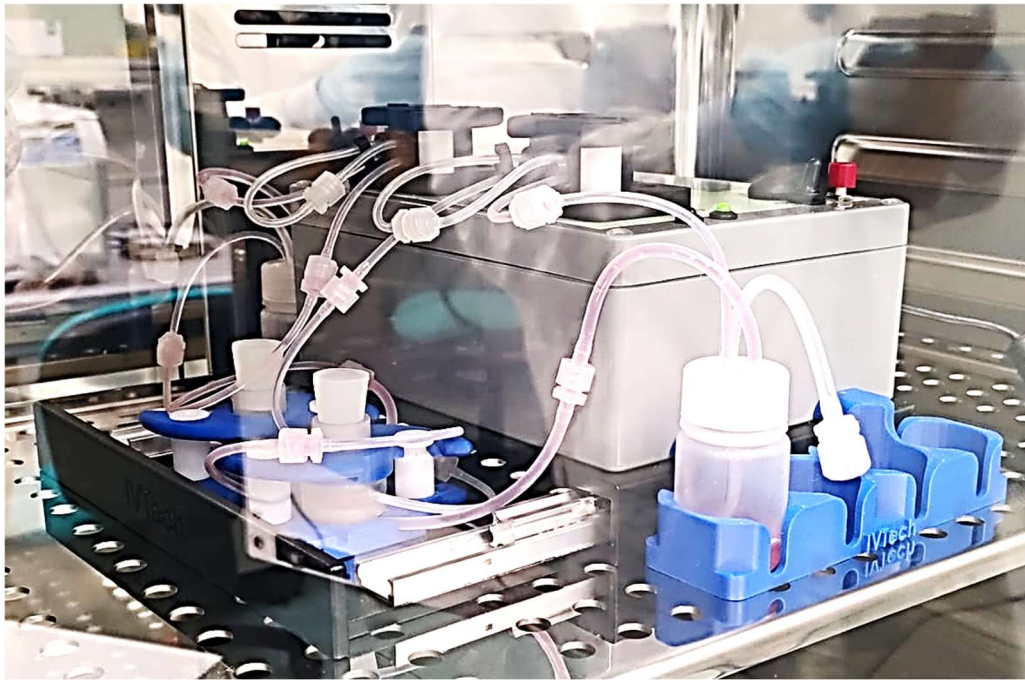
Figure 26 – Experimental human skin mode in dynamic condition. The skin sample was cultured in culture chamber. The epidermis and wound area was exposed to the air
