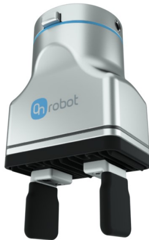
Figure 3.7: OnRobot 2FG7 electric finger gripper [69]
