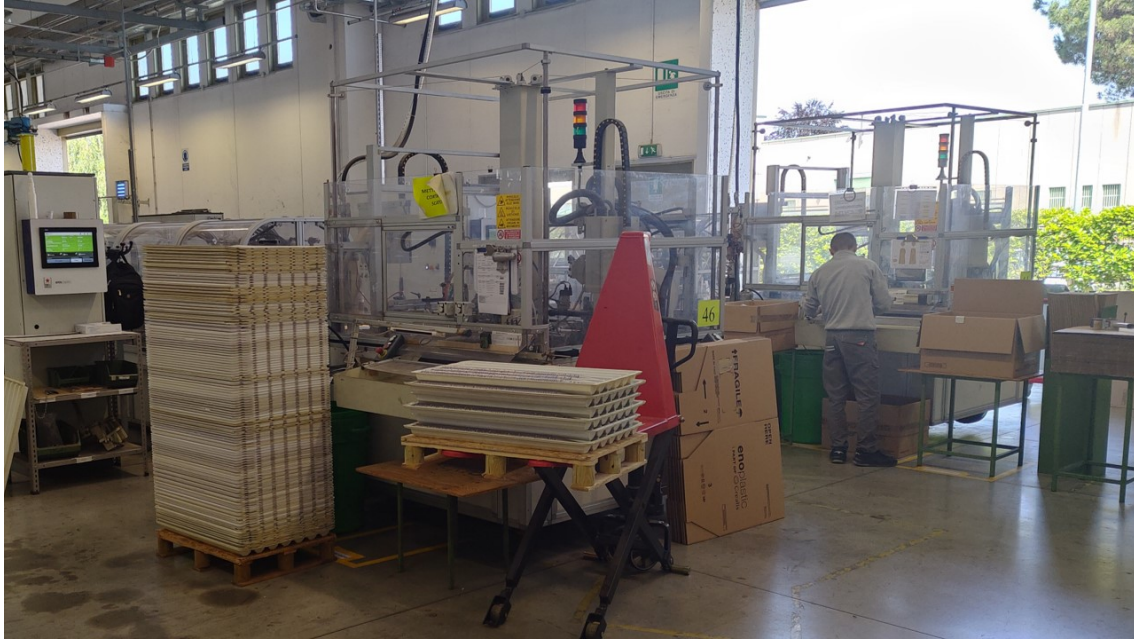
Figure 5.2: Manual setup of unloading cells. In the foreground is visible the pallet of empty trays on the left, and on the right the corresponding output stack of trays to be filled with the products deposited in the central buffer collector of the machine. In the background, the operator unloads the second machine with similar characteristics.
