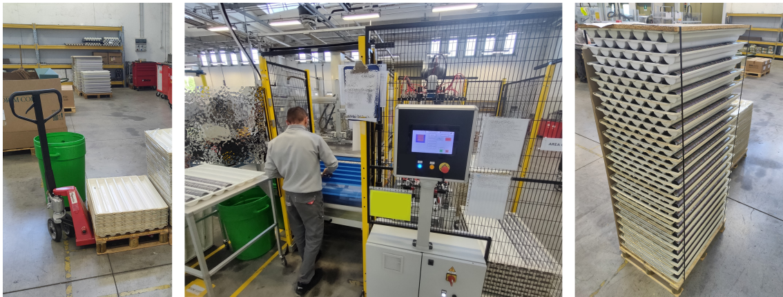
Figure 5.10: Operator's duties after implementing the robotic unloading cell. The operator is required to supply the pallets of empty trays to the robotic cell (left), supervise the starting phase of the machine, thus checking the quality compliance to the requisites of the products being produced by the automatic machine (center), and prepare the output stack of trays for shipment (right).
