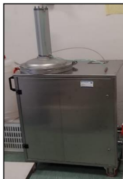
Figure 25. Solid-liquid Naviglio® extractor based on cyclic pressurization phases.
