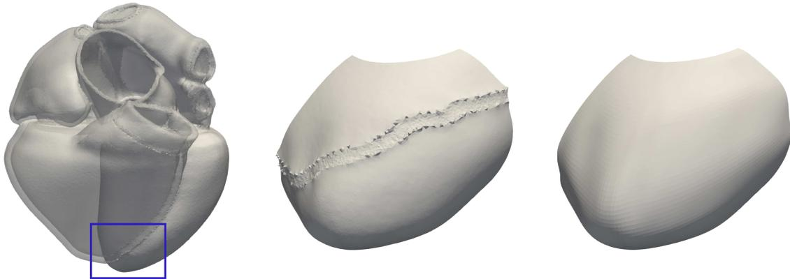
Figure A.2: Artifacts generated during the extraction of the selected surface from the four-chamber geometry.
