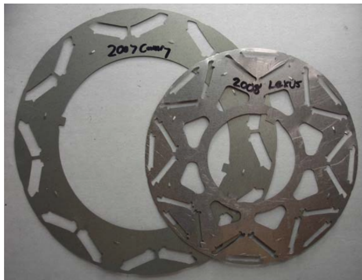
Figure 1.3: Comparison of motor rotor laminations, Toyota Camry (left) vs. Lexus LS 600H (right) [5].
