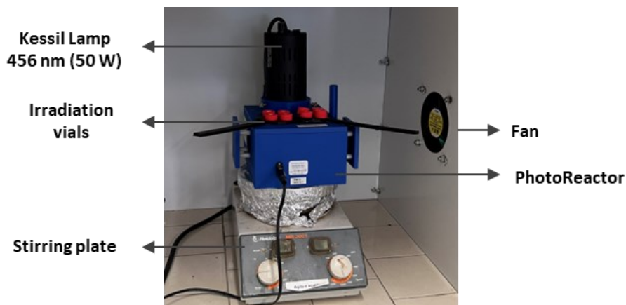
Figure ES6.4. Irradiation set up for the one-pot protocol in batch.
