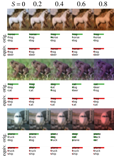
Figure 5.5: Comparison of the predictions obtained on three images taken from the CIFAR-10 test set. Each image has been distorted by the introduction of an artificial illuminant with saturation varying from 0.0 (no distortion) to 0.8. The top three classes predicted by the original and the equivariant ResNet-20 are reported below each image. The lengths of the bars is proportional to the posterior probabilities estimated by the networks.
